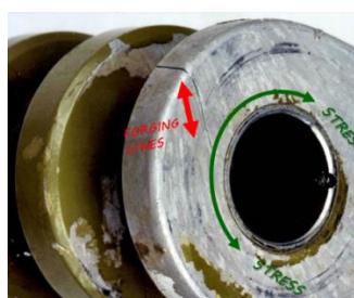
4.b: Another example of stress corrosion that could be tested. Forging lines drive crack direction.
