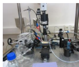
Figure 2.b, reprint from [12]. Glass micro electrodes used to measure pH and potential of the electrolyte at edge of a defect in a PPG PAC 33 polyurethane coating. A mass transport model solved with FEM was used to deduce Cr(VI) ion concentration gradients during release.
