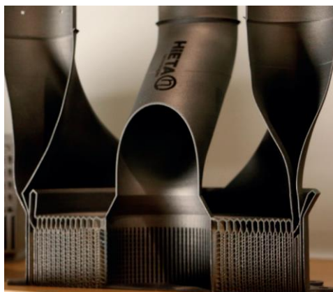
Figure 1: Selective Laser Melting of Micro Turbines recuperator
